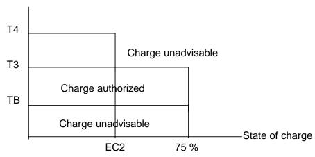
If the temperature exceeds these limits during charging, the charge must be interrupted and restarted only when the temperature has dropped to the authorised fast charge temperature.
