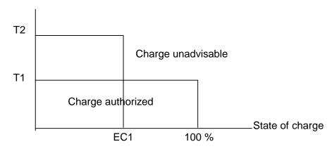
The authorised T1 temperature value of +40°C must not be considered as a value to start the charge systematically. Actual module temperature around +30°C is strongly recommended in order to guarantee the life time and the performance of the battery.
