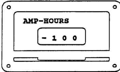
AMP-HOUR meter counts Amp-hours (Ahrs) used from the battery and displays them with a minus sign. When charging begins, Ahrs are added until the display reads 0 when the battery is fully charged. Overcharging will continue to add Ahrs and they will be displayed as a positive number. When discharging begins from the overcharge state, AMP-HOUR meter automatically resets to 0 and starts counting down as Ahrs are used.
