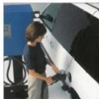
▲ Right where it should be, the charging point is located in the same location as the fuel fill on a gasoline-powered minivan.
