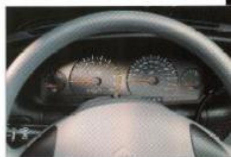
▲ The instrument cluster features a state-of-charge gauge which calculates the charge remaining in the battery system.
