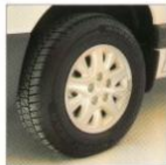
▲ Low rolling resistance tires reduce road friction.
