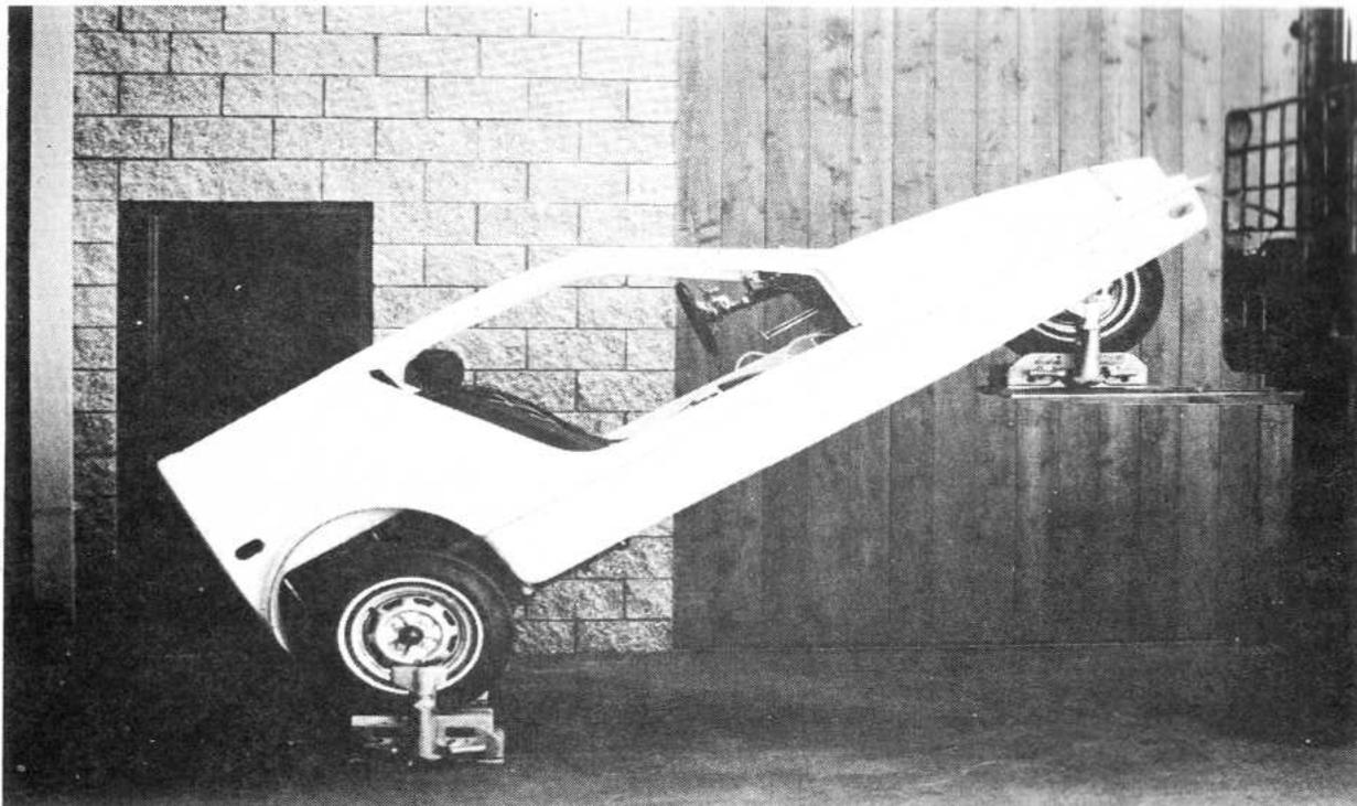
Fig. 8 Measurement of the Center of Gravity Location by Taking Wheel Weights in Different Positions
