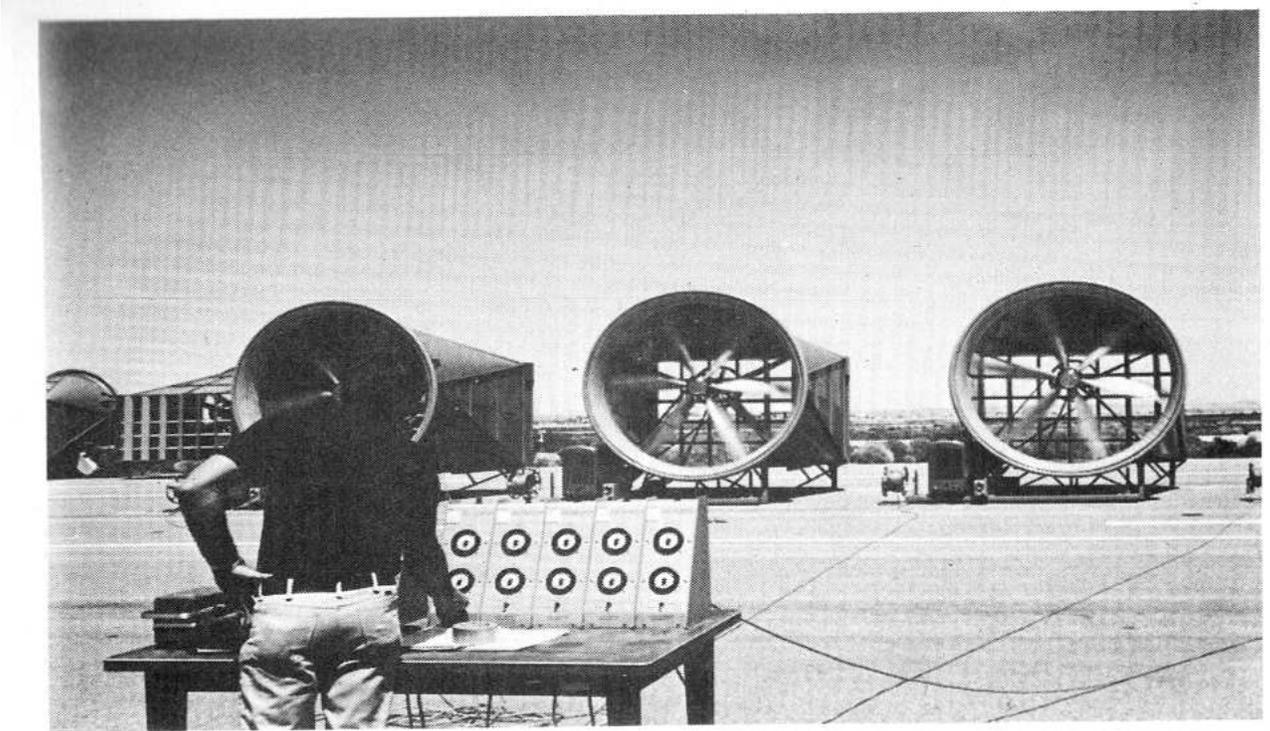
Fig. 6 Three of Eight Units of the NHTSA Crosswind Generator
