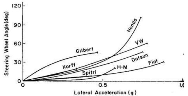
Fig. 13 Understeer Curves for All Test Cars
