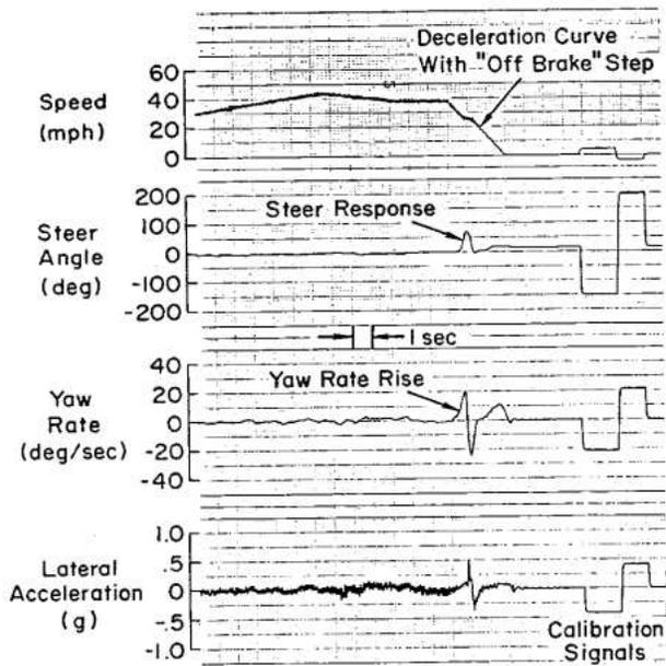
Fig. 10 Example of Strip Chart Data, Straight Brake with Rear Lockup
