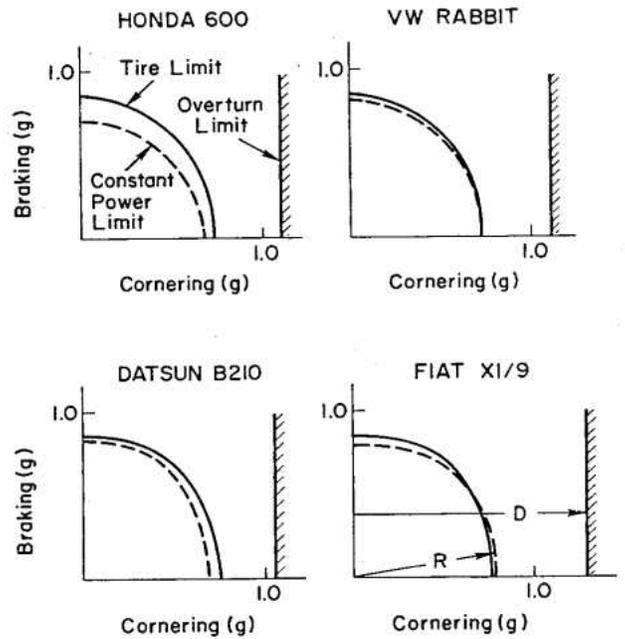
Fig. 11 Prediction of Overturn Limits for 4-Wheeled Vehicles
