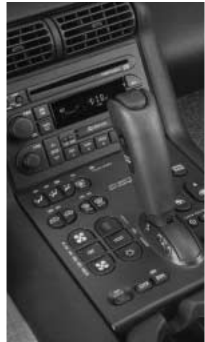
Console Control Unit consolidates most controls in one central module.
