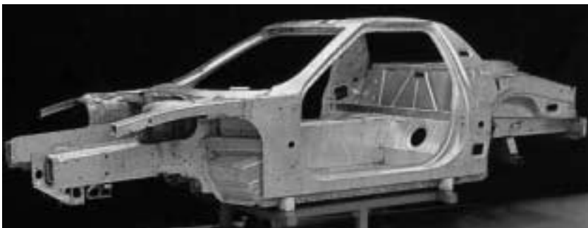
The EV1's bonded and welded aluminium spaceframe.
