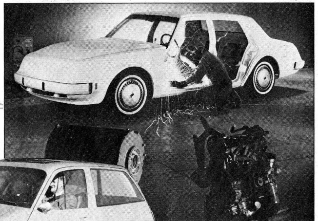
Hybrid car being built by GE (above) uses a 45-hp electric motor and a 75-hp gasoline motor, running on either or both as necessary. At left is GE's test vehicle built with off-the-shelf components.
