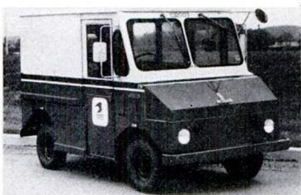
Batronic minivan is built on a 6400-lb. GVW chassis, and powered by two 48V
