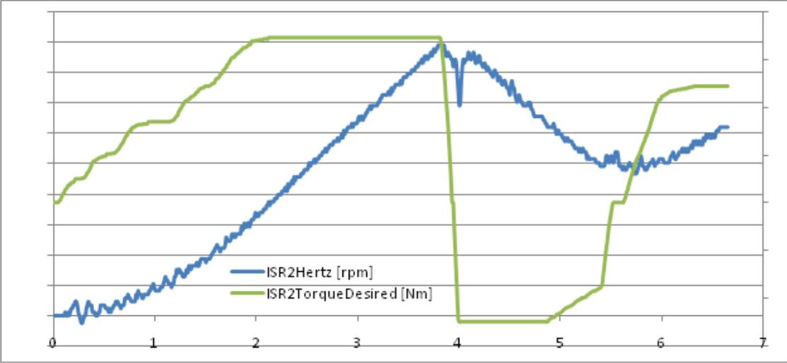
Figure 18: Example Torque Step Test Results With Damping Enabled
