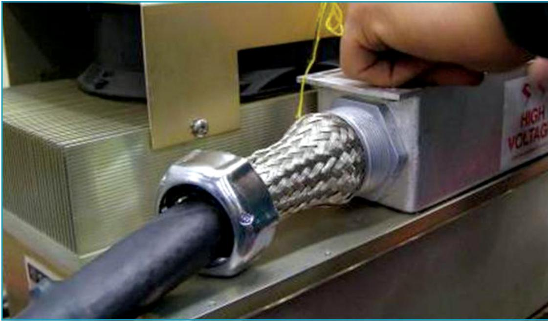
Figure 26: DMOc445 Motor Power Cable Entrance, 360° Shielding
