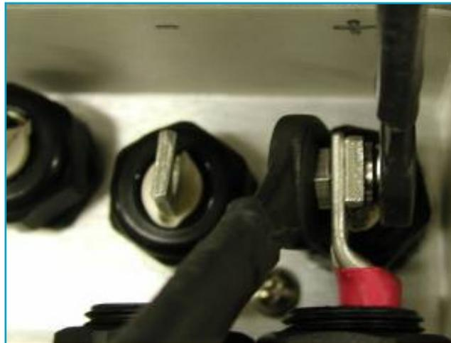
Figure 22: DMOC445 Motor Power Wire Connections
