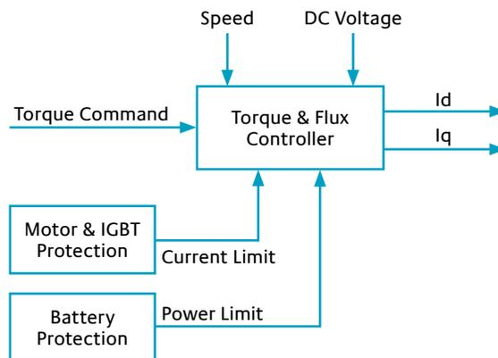
Figure 15: Torque Controller with Protections
