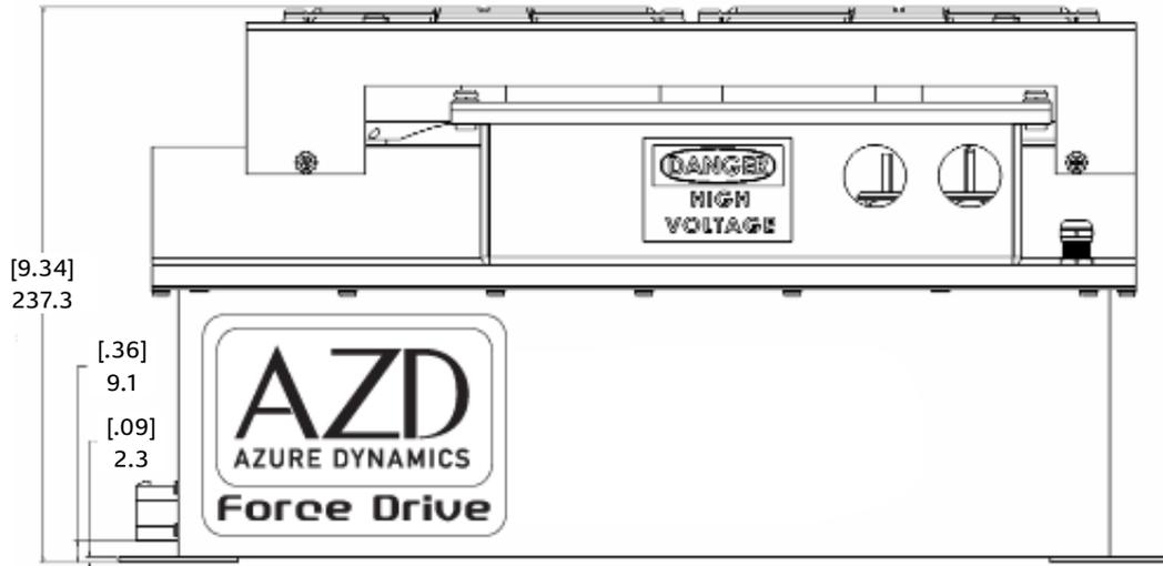
Figure 5: DMOc445 Air-Cooled Dimensions, Side View
