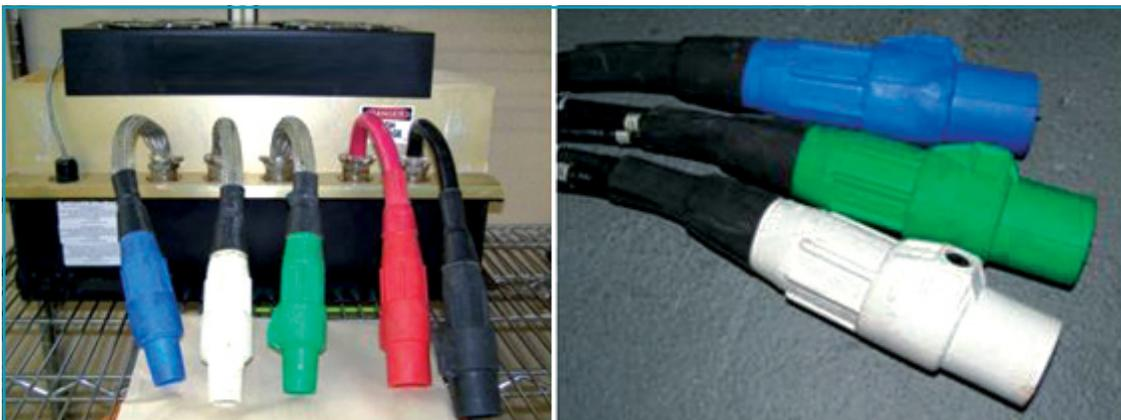
Figure 32: DMOC645 High Voltage Cables with Cam-Lok Connectors and AC90 Motor Power Cables
