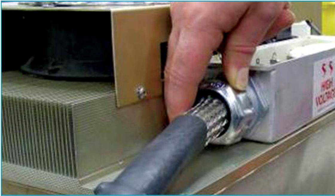
Figure 28: DMOC445 Motor Power Cables Grommet
