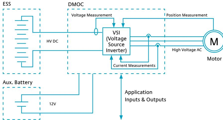
Figure 2: DMOC with Typical Connections
