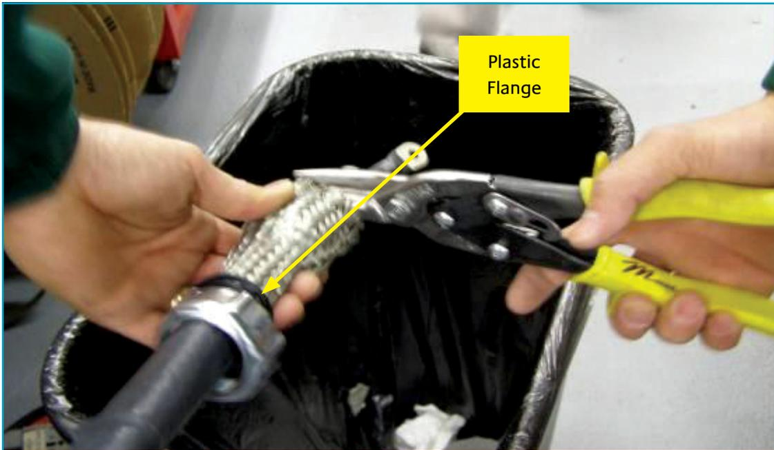
Figure 29: DMOC445 Motor Power Cable Black Plastic Flange Washer
