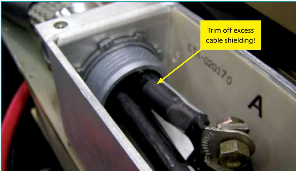
Figure 27: DMOc445 Motor Power Cable, Trim Shielding
