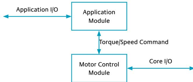
Figure 1: DMOC Application Module and Control Core
