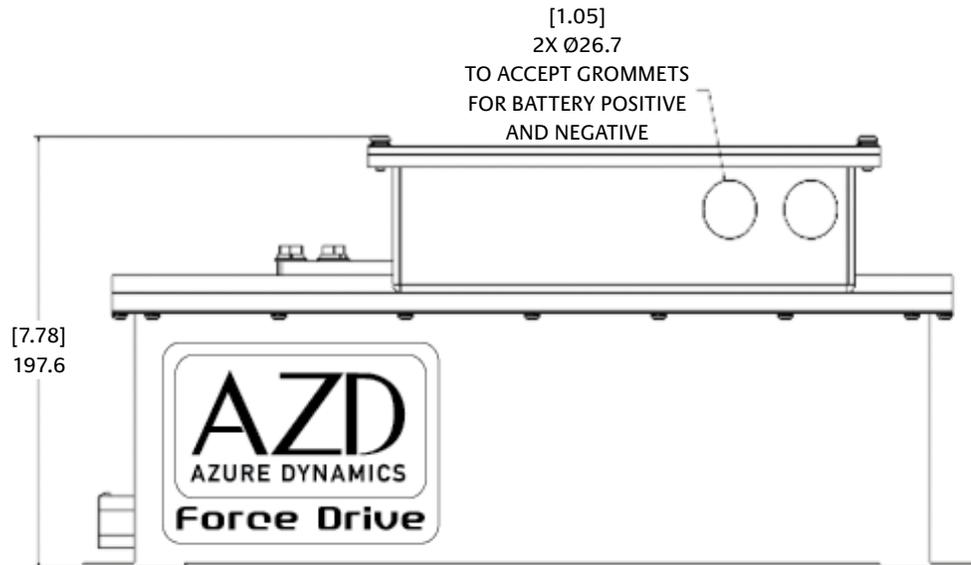
Figure 10: DMOC445 Battery Wire Connections
