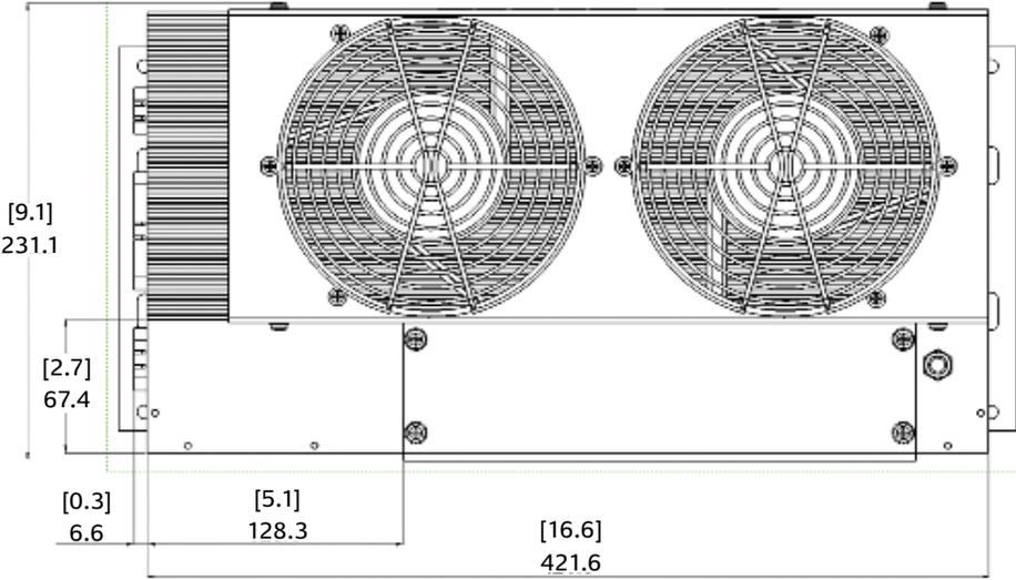
Figure 4: DMOC445 Air-Cooled Dimensions, Top View
