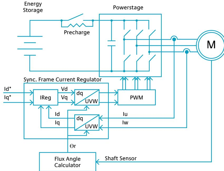
Figure 14: Synchronous Frame Current Regulator
