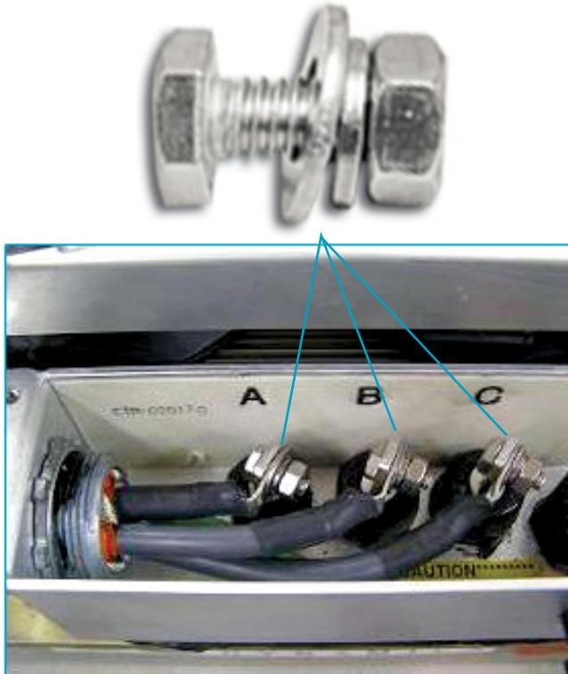
Figure 23: DMOc445 Motor Connection Hardware and Terminals
