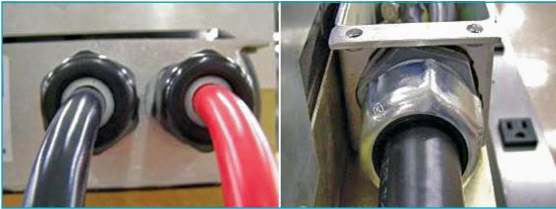
Figure 31: DMOCC445 Battery Cable and Motor Cable Fittings
