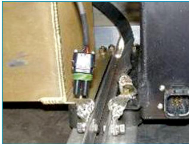
Figure 34: Example DMOC Grounding Strap Connection
