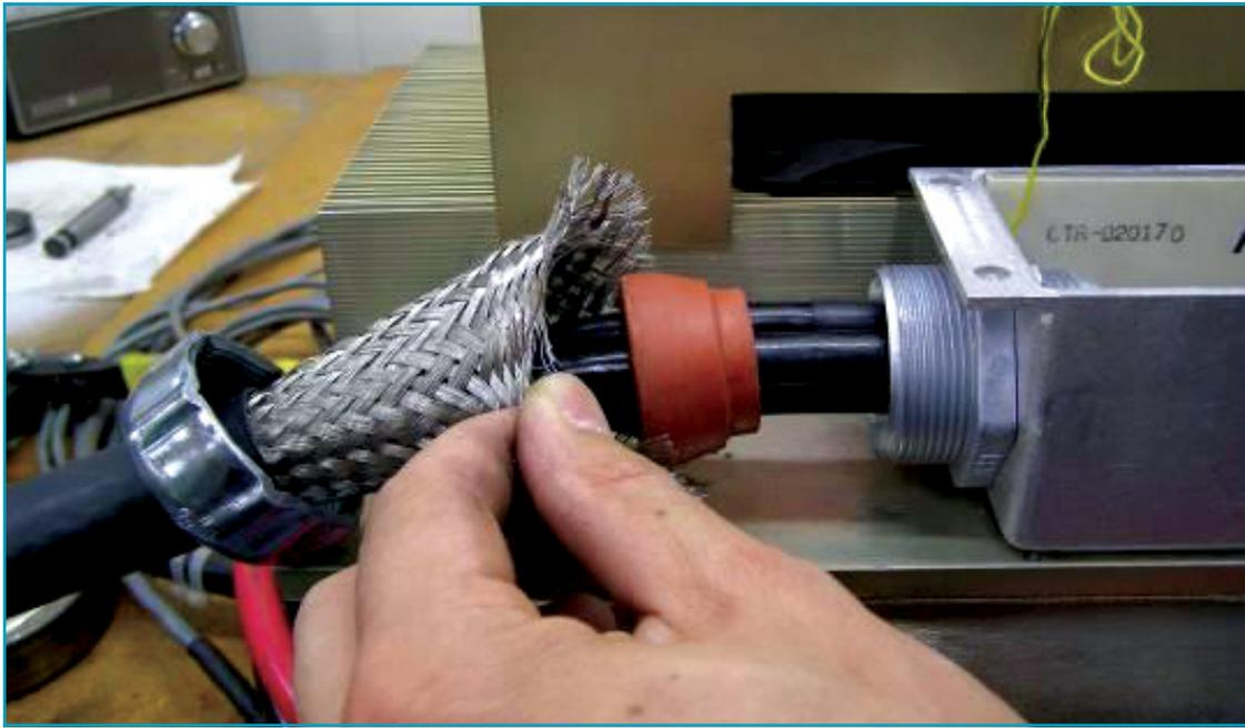
Figure 24: DMOC445 Motor Power Cable Entrance Fitting
