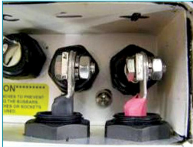
Figure 30: DMOC445 High Voltage Battery Terminals
