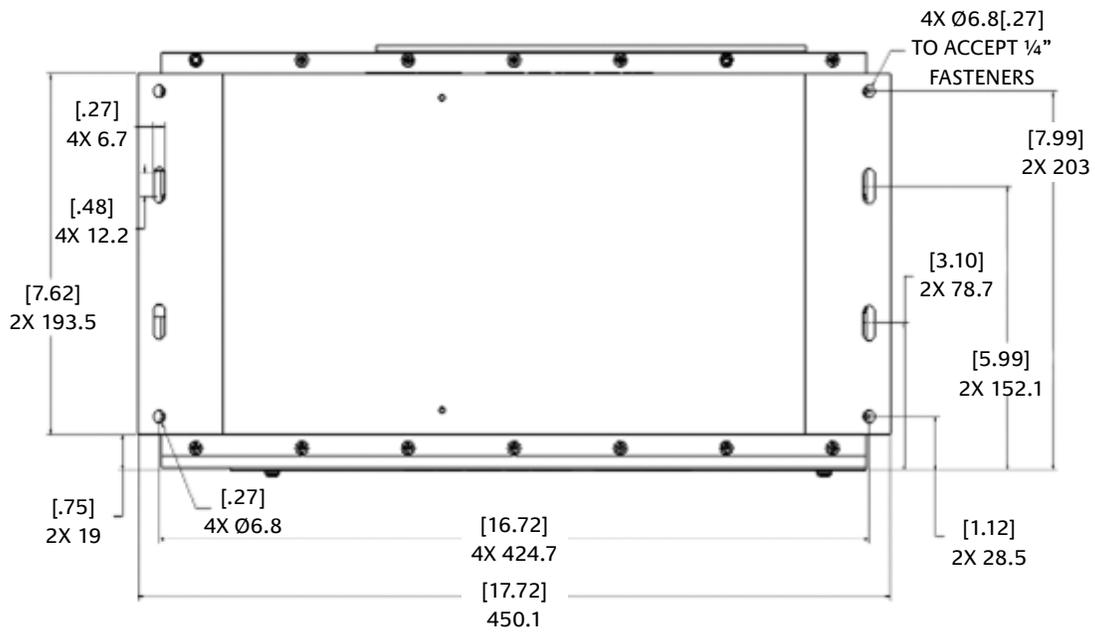
Figure 7: DMOC445 Dimensions, Bottom View
