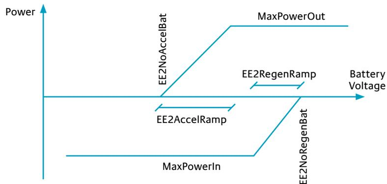
Figure 16: Battery Protection
