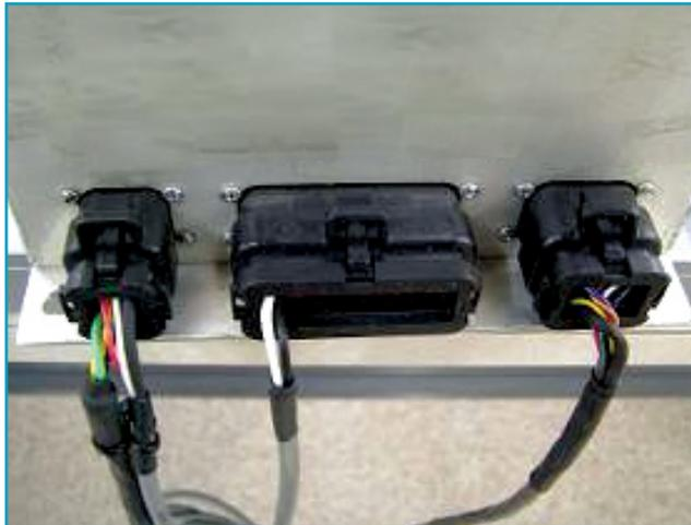
Figure 20: All three DMOC connectors in position
