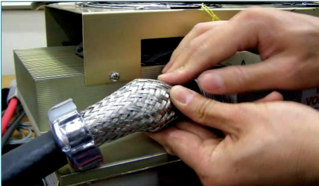
Figure 25: DMOC445 Motor Power Cable Shielding
