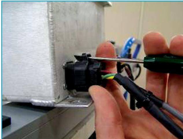
Figure 19: Removing 8-Pin Communications Connector
