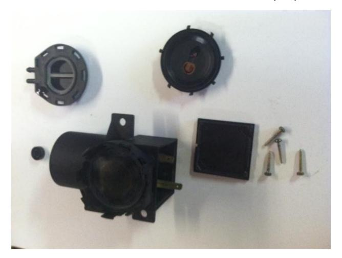
The pump is serviceable for oiling and freeing up the rotor if it does not rotate.
