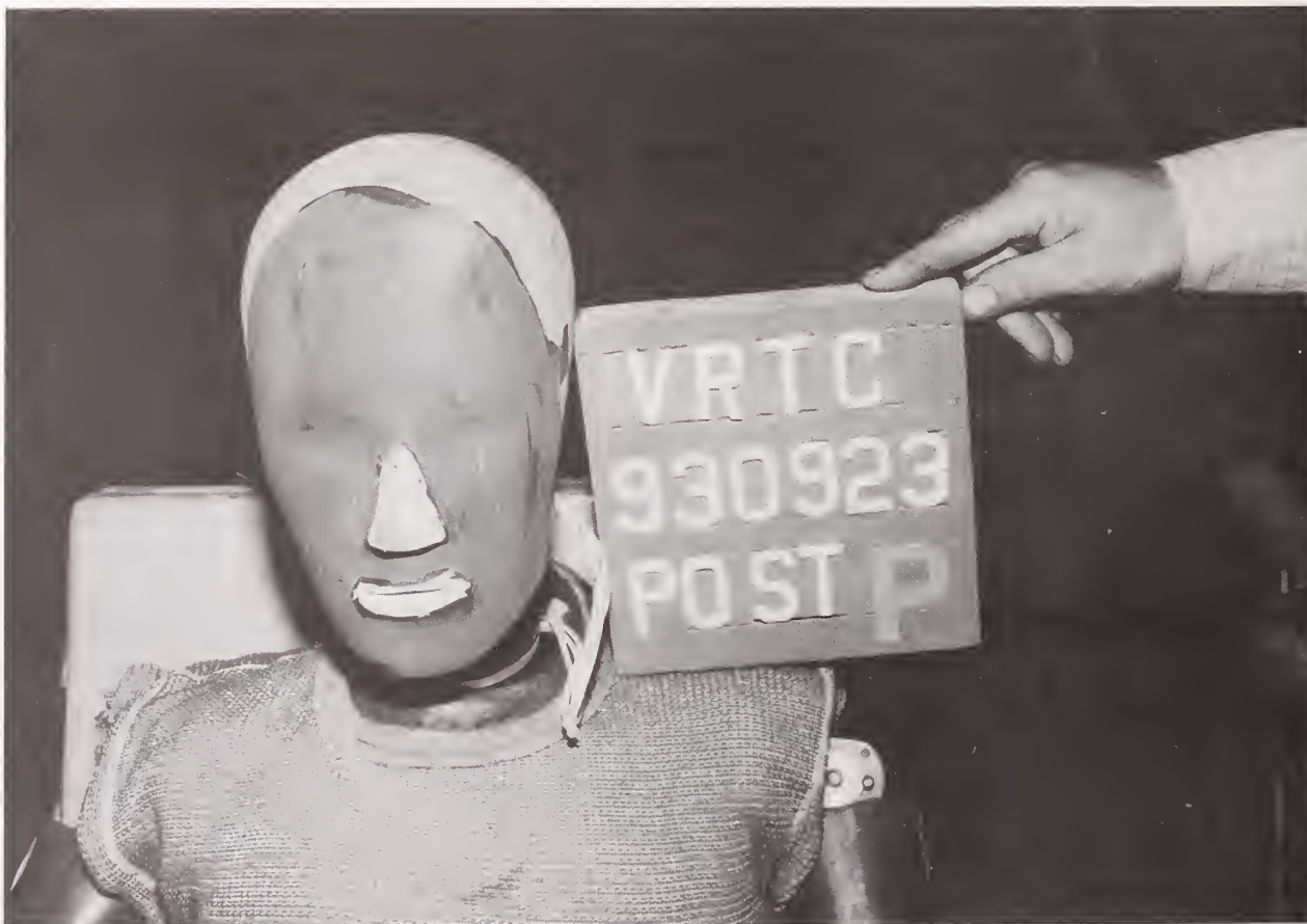
Figure A-40. POST-TEST PASSENGER DUMMY HEAD CONTACT - VIEW 1
