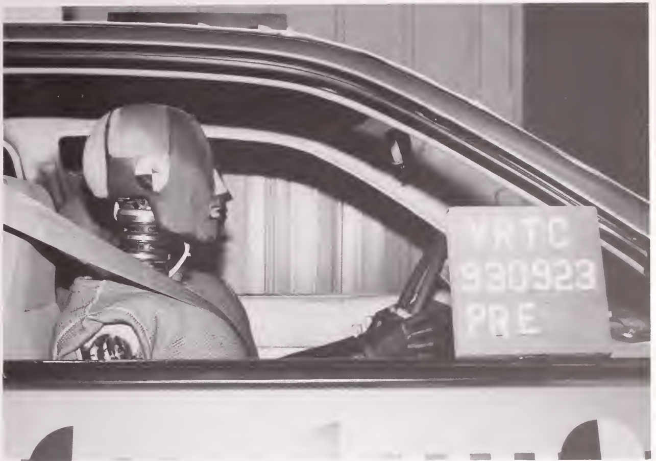
Figure A-25. PRE-TEST PASSENGER DUMMY POSITION VIEW
