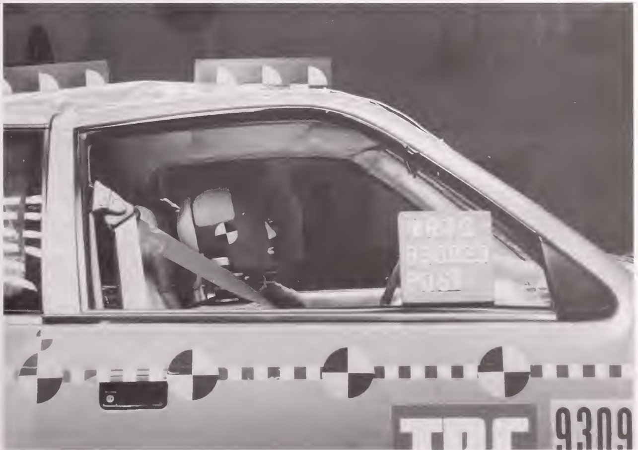
Figure A-26. POST-TEST PASSENGER DUMMY POSITION VIEW
