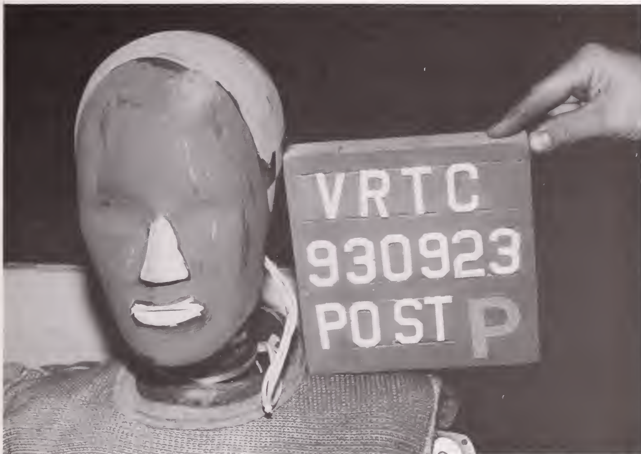
Figure A-41. POST-TEST PASSENGER DUMMY HEAD CONTACT - VIEW 2
