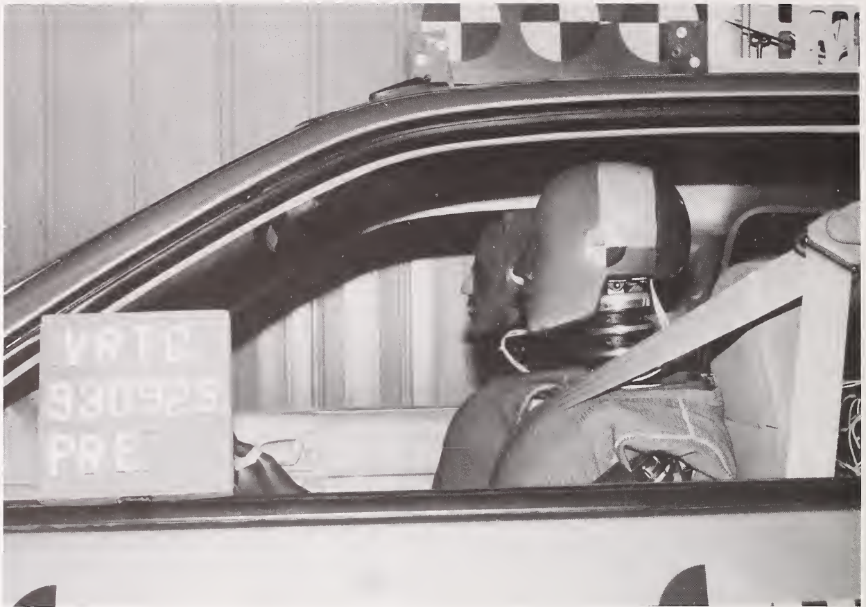
Figure A-23. PRE-TEST DRIVER DUMMY POSITION VIEW
