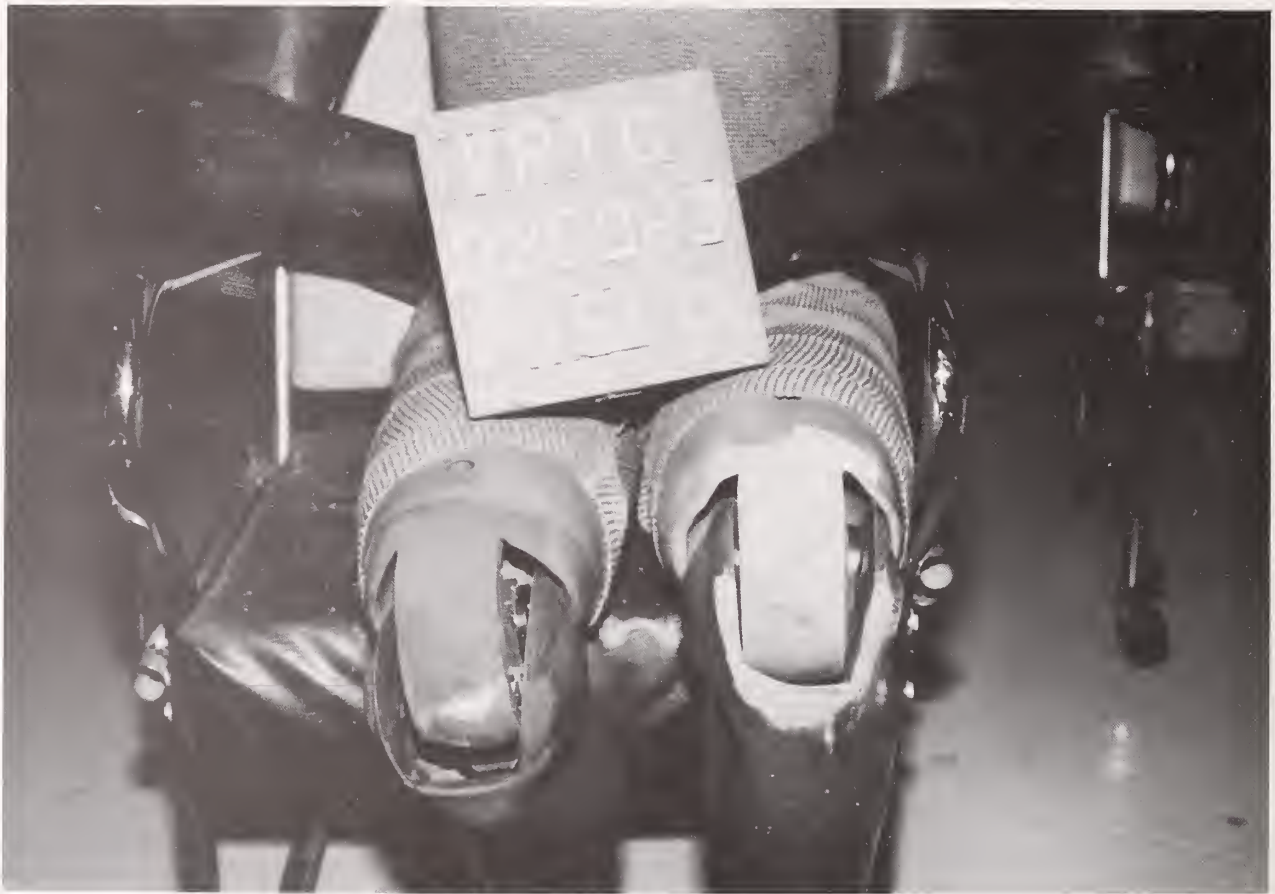
Figure A-43. POST-TEST PASSENGER DUMMY KNEE CONTACT - VIEW 1
