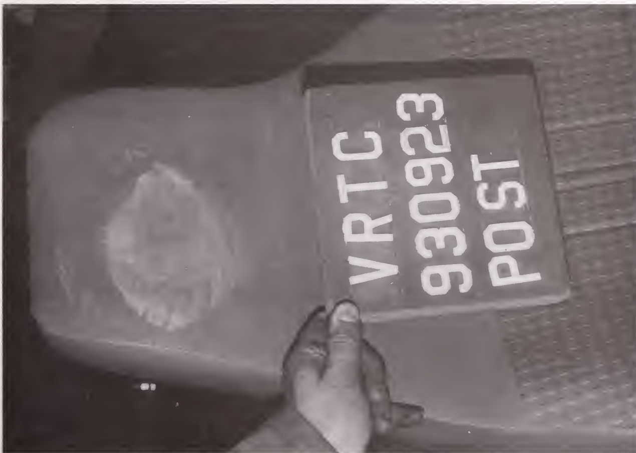
Figure A-42. POST-TEST PASSENGER DUMMY HEAD CONTACT - VIEW 3
