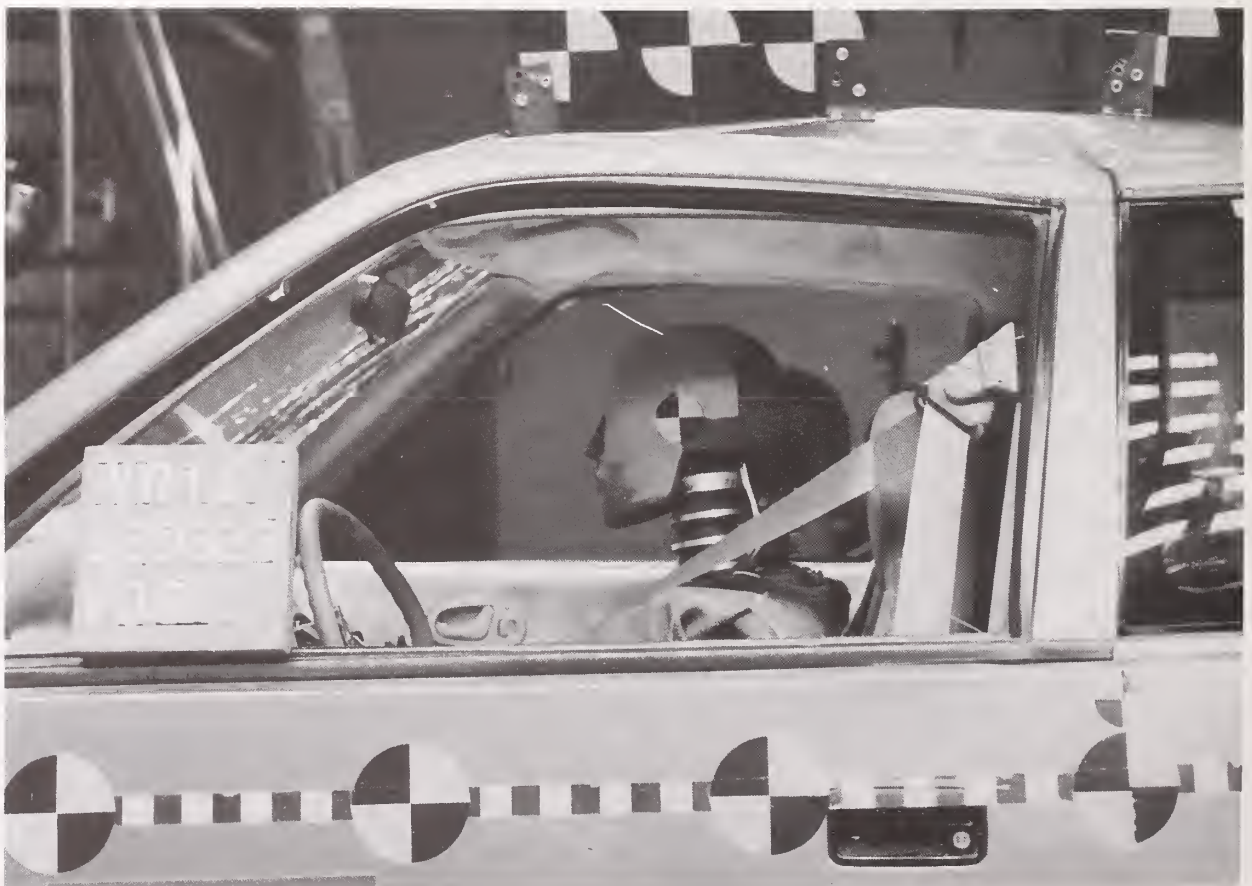
Figure A-24. POST-TEST DRIVER DUMMY POSITION VIEW
