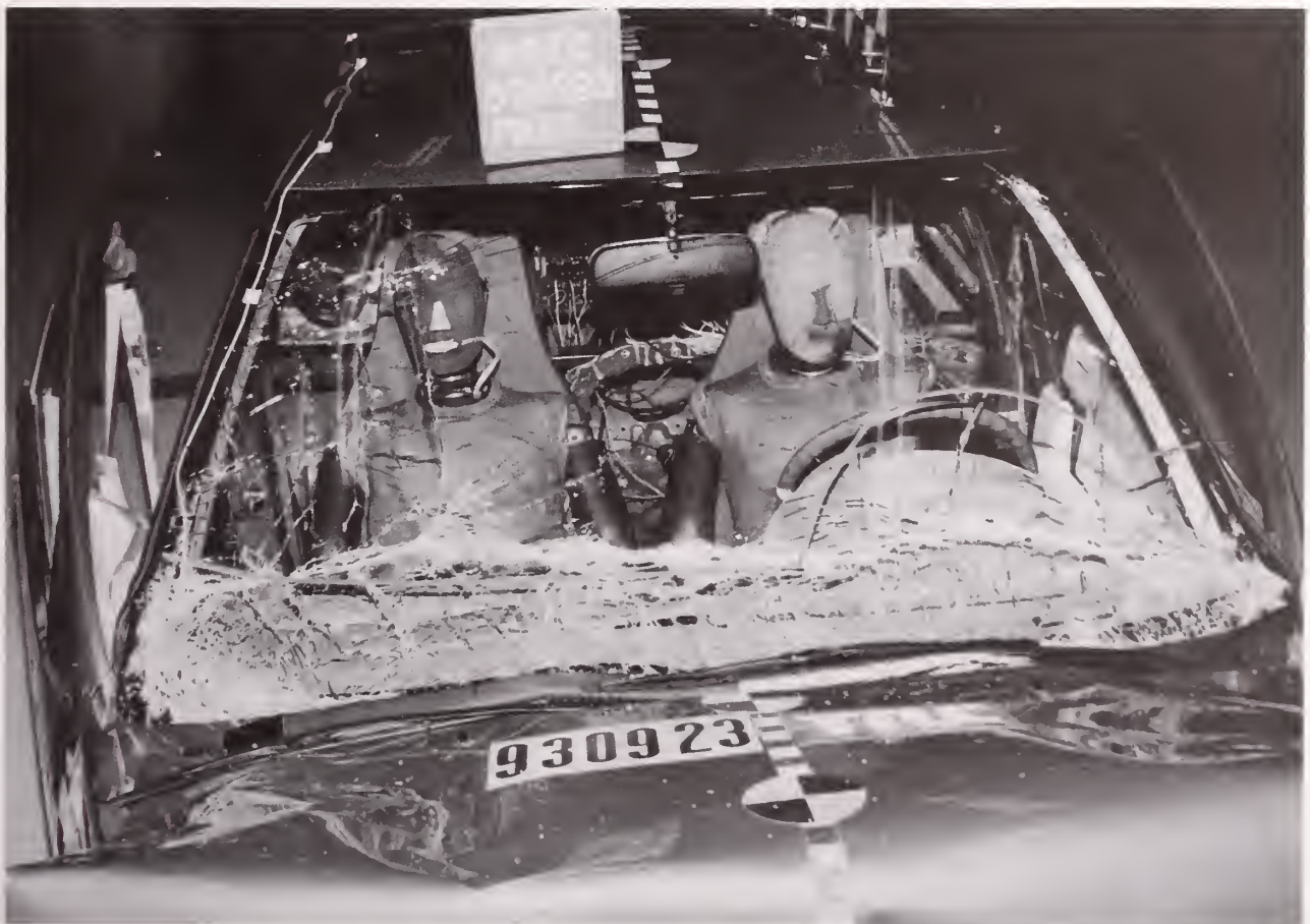
Figure A-14. POST-TEST WINDSHIELD VIEW
