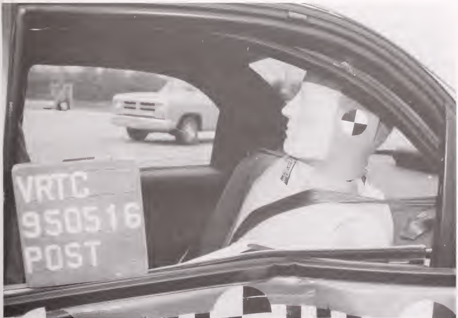
Figure A-19 Pre-test Passenger Dummy Position View
