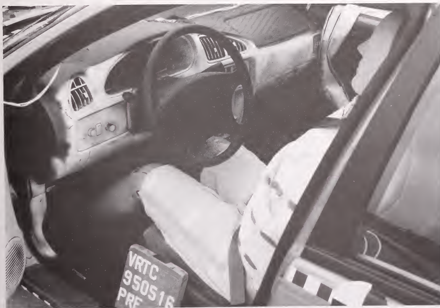
Figure A-16 Pre-test Driver Dummy and Vehicle Interior - View 1
