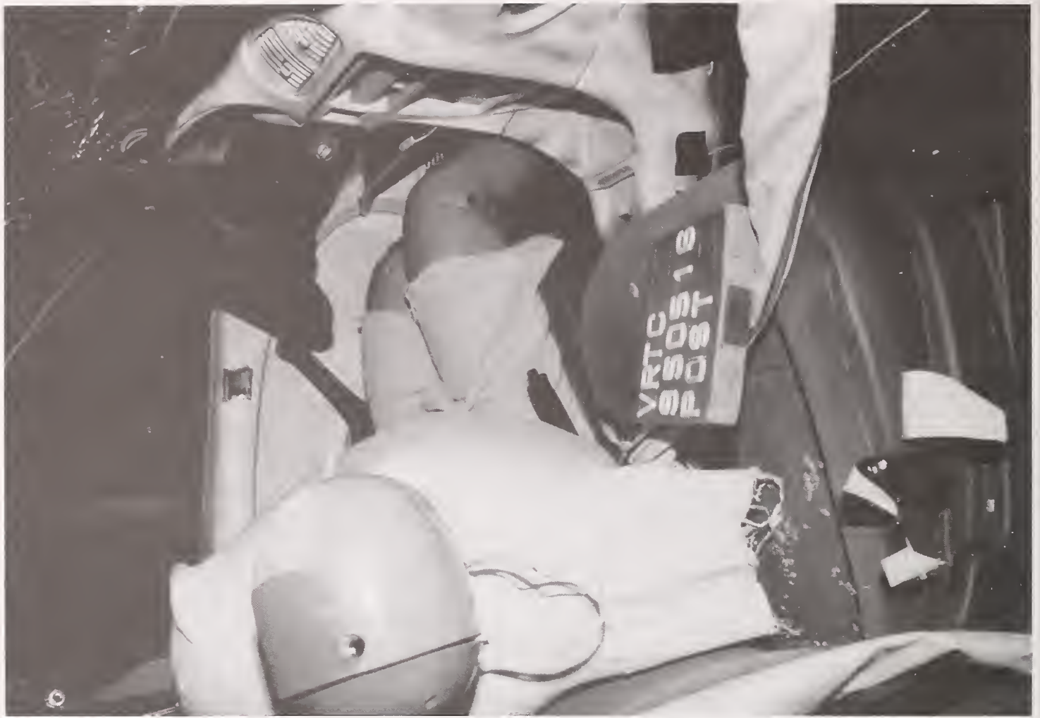
Figure A-18 Post-test Driver Dummy and Vehicle Interior View
