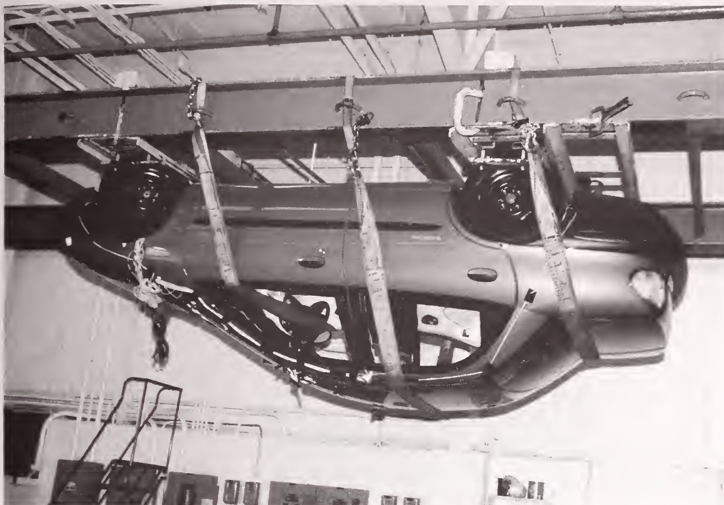
Figure A-32 Post-test Vehicle on Static Rollover View
