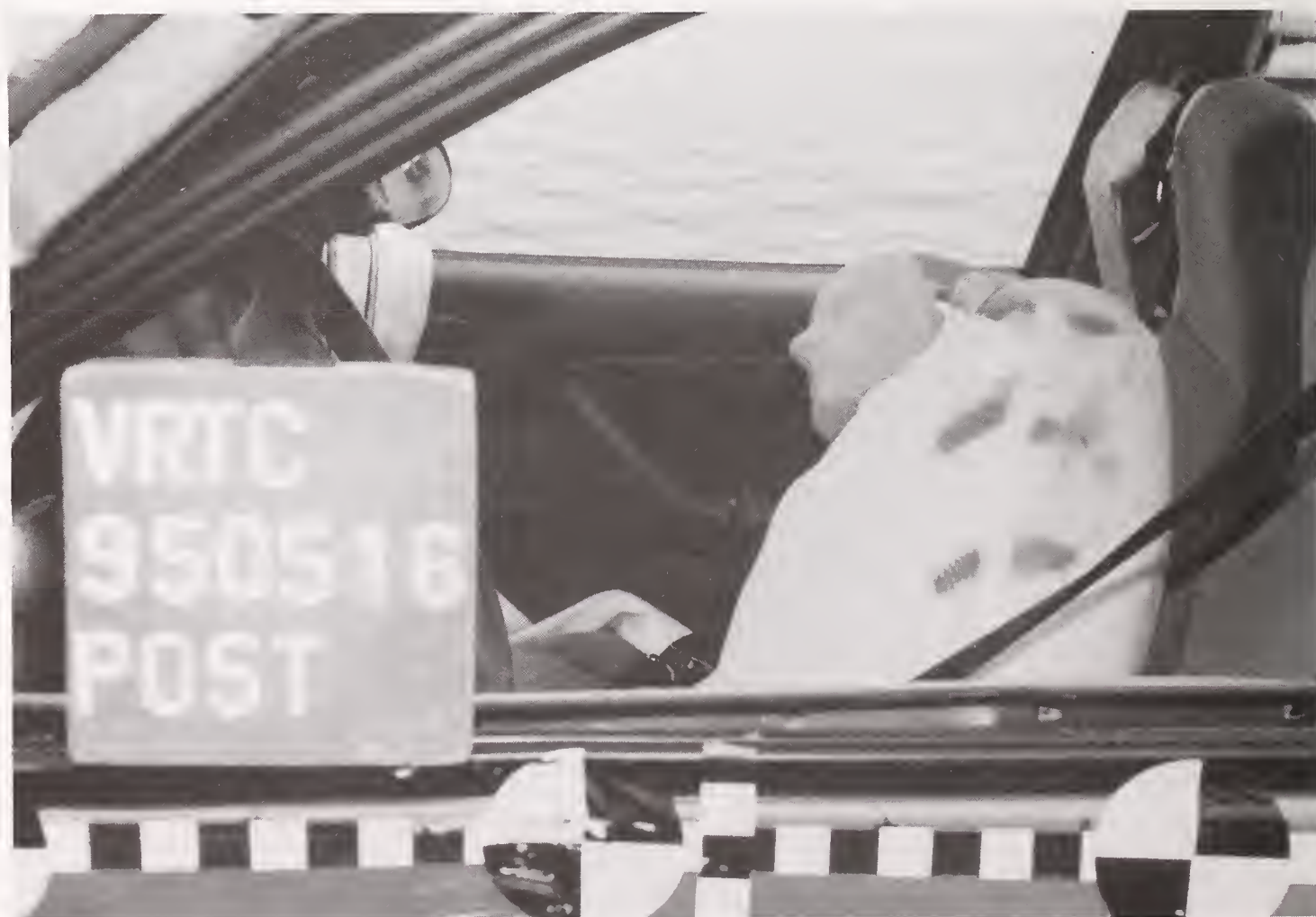
Figure A-15 Post-test Driver Dummy Position View
