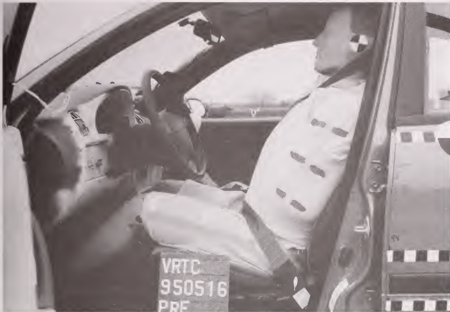
Figure A-16 Pre-test Driver Dummy and Vehicle Interior - View 1
