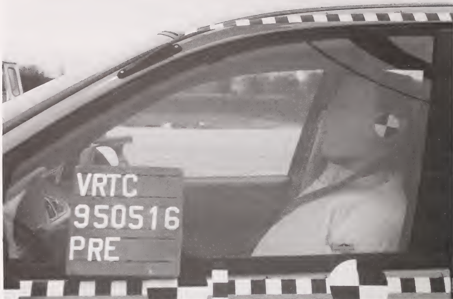
Figure A-14 Pre-test Driver Dummy Position View
