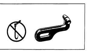
Always use "T"-hooks inserted into the "T"-hook slots. See diagrams.
