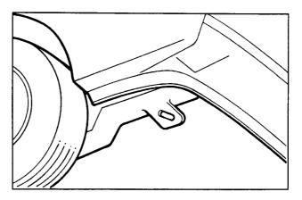
Attach T-hook chains on both sides, in the slotted holes in the brackets, just ahead of the front wheels.
