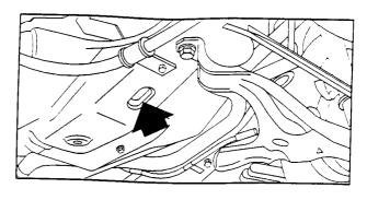
Attach T-hook chains to the T-hook slots in the bottom of the floor pan just ahead of the rear wheels on both sides.
